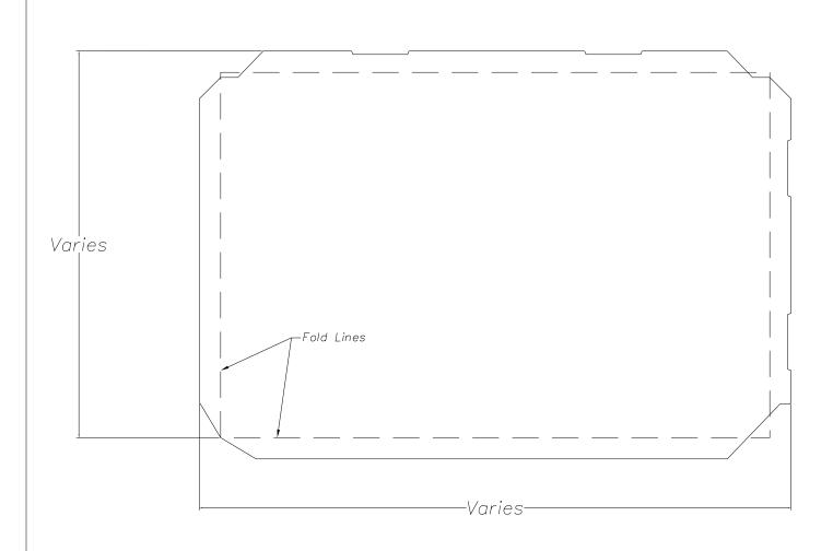
NOTE: Recommended fastener is MT100 Clip. Spacing is dertermined by project.Panel above is shown as a left to right install.
