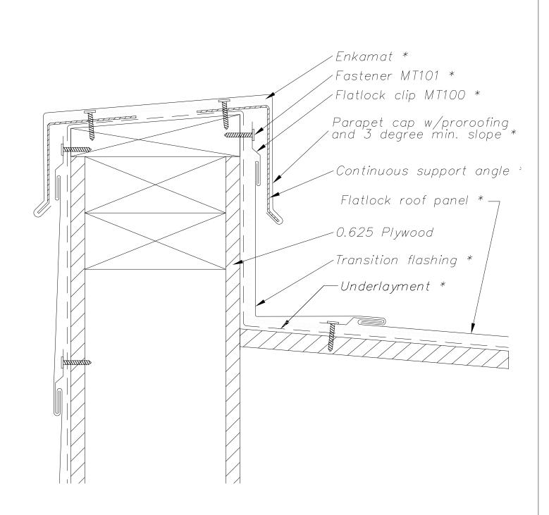
DRAWING NAME: PARAPET DETAIL - OPTION 1 REVISION NO:
