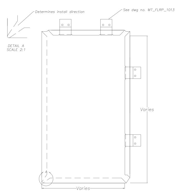
NOTE: Recommended fastener is MT100 Clip. Spacing is dertermined by project. Panel above is shown as a left to right install.
