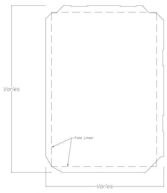
NOTE:Recommended fastener is MT100 Clip. Spacing is dertermined by project.Panel above is shown as a left to right install.
