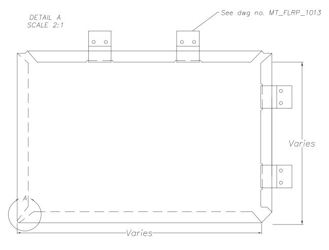
NOTE:Recommended fastener is MT100 Clip. Spacing is dertermined by project.Panel above is shown as a left to right install.
